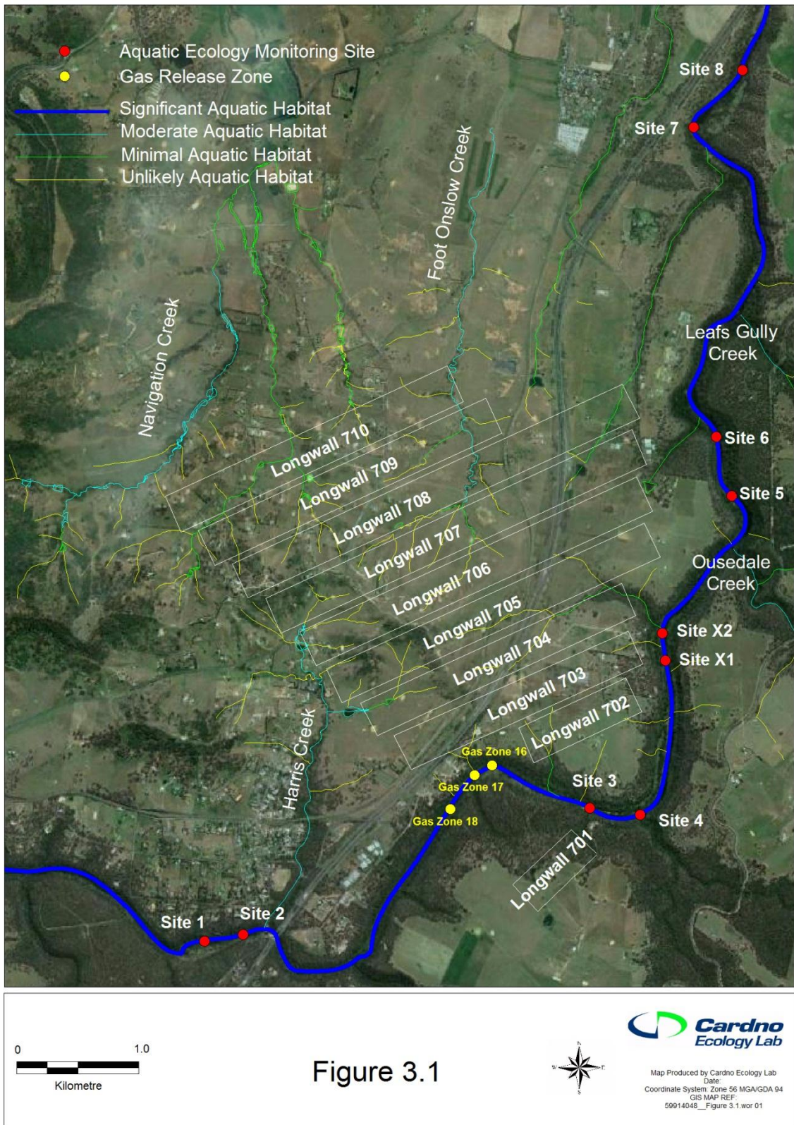
Figure 6-3: Aerial photograph of the study area showing aquatic ecology monitoring sites and gas release zones identified during extraction of Longwall 705, CEL (2014).
