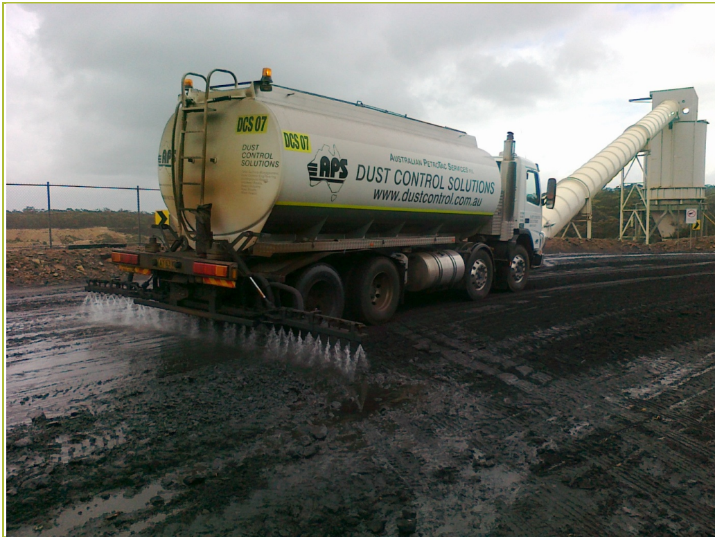
Figure 3.1 Suppressant trial on haul roads at West Cliff
