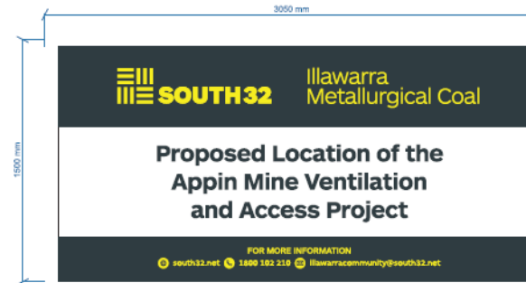
ACP PANEL DIGITALLY PRINTED + UV LAMINATED GRAPHICS APPLIED TO FACE
