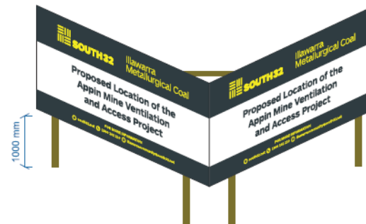
X4 125mm TREATED PINE COPPER LOGS 800mm CONCRETE EMBEDEDMENT 45 x 90mm TREATED PINE FRAMEWORK BEHIND SIGN PANELS + BRACING
