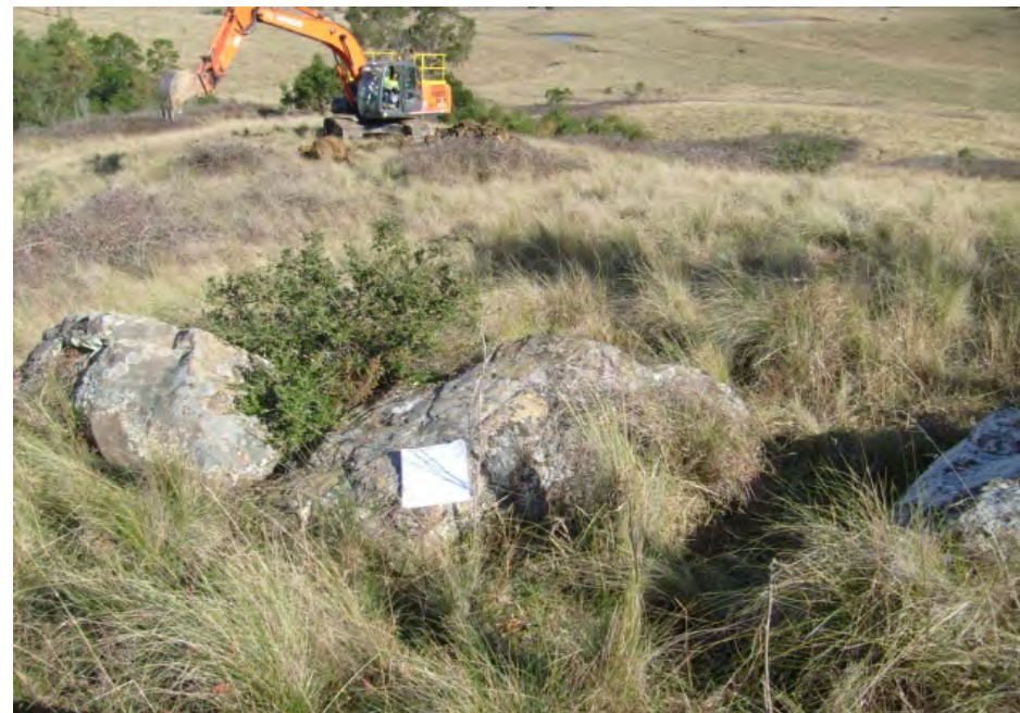
Large Boulders on Surface Part of Colluvium on Lower Part of Landslide
