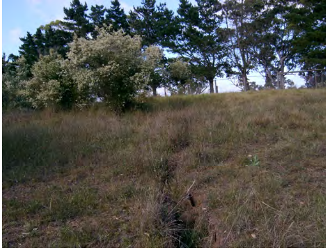
Fig. 4.13 Surface Tension Cracking along the Top of a Steep Slope
