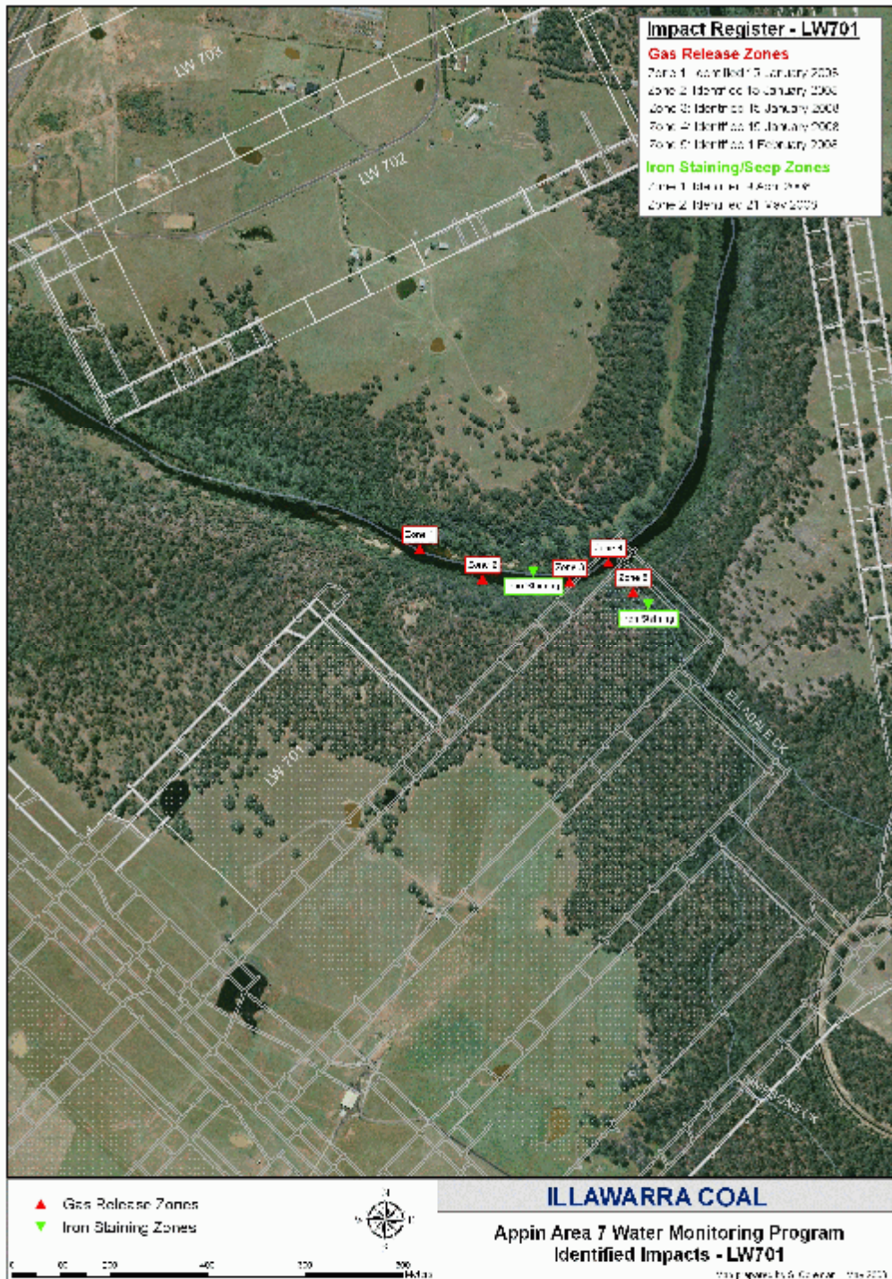
Figure 2.15 Gas Emissions and Iron Staining Zones in Nepean River Near Longwall 701
