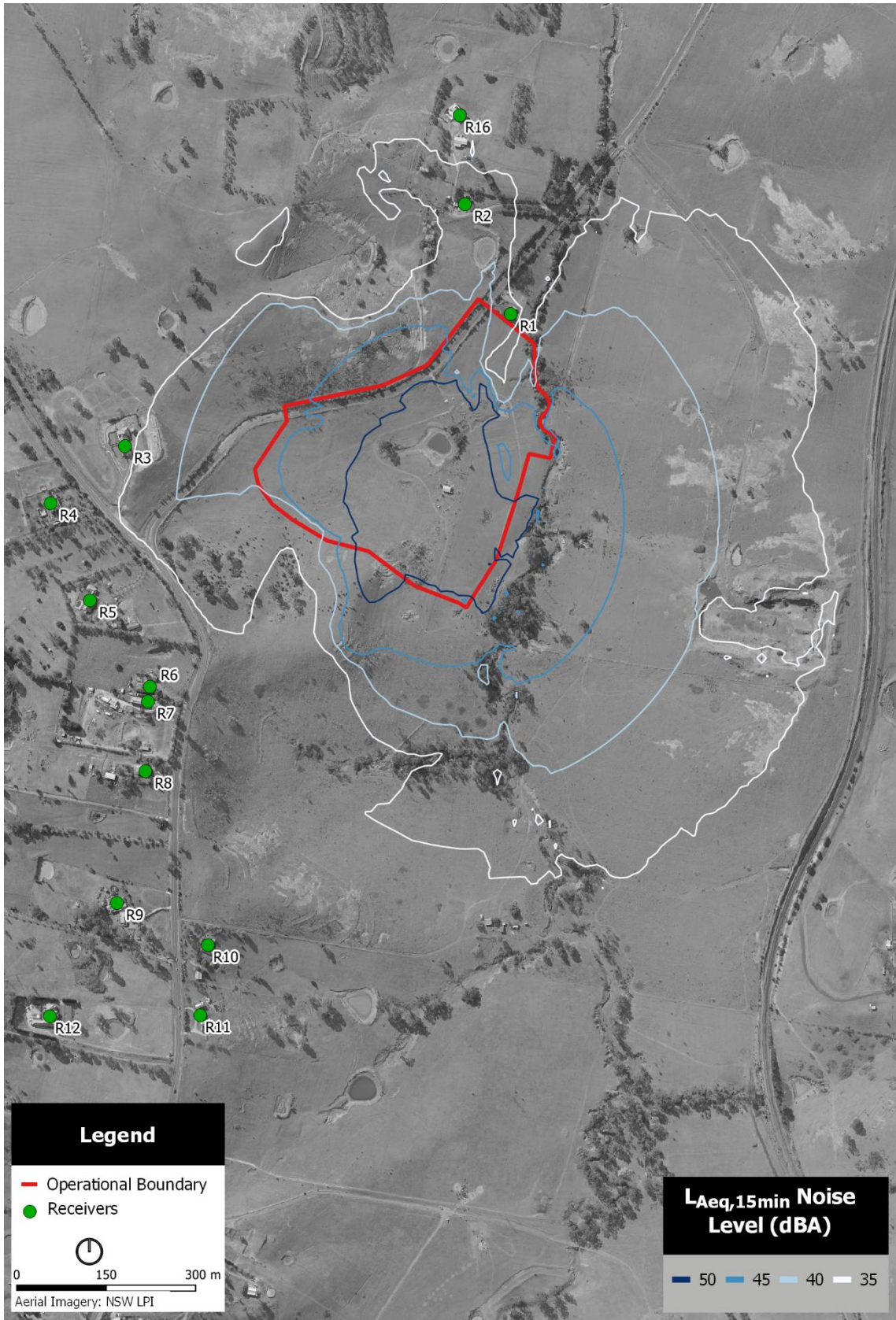
Figure 11 Predicted Night Noise Levels - Ventilation Fans and Mine Access, Noise-enhancing Meteorology
