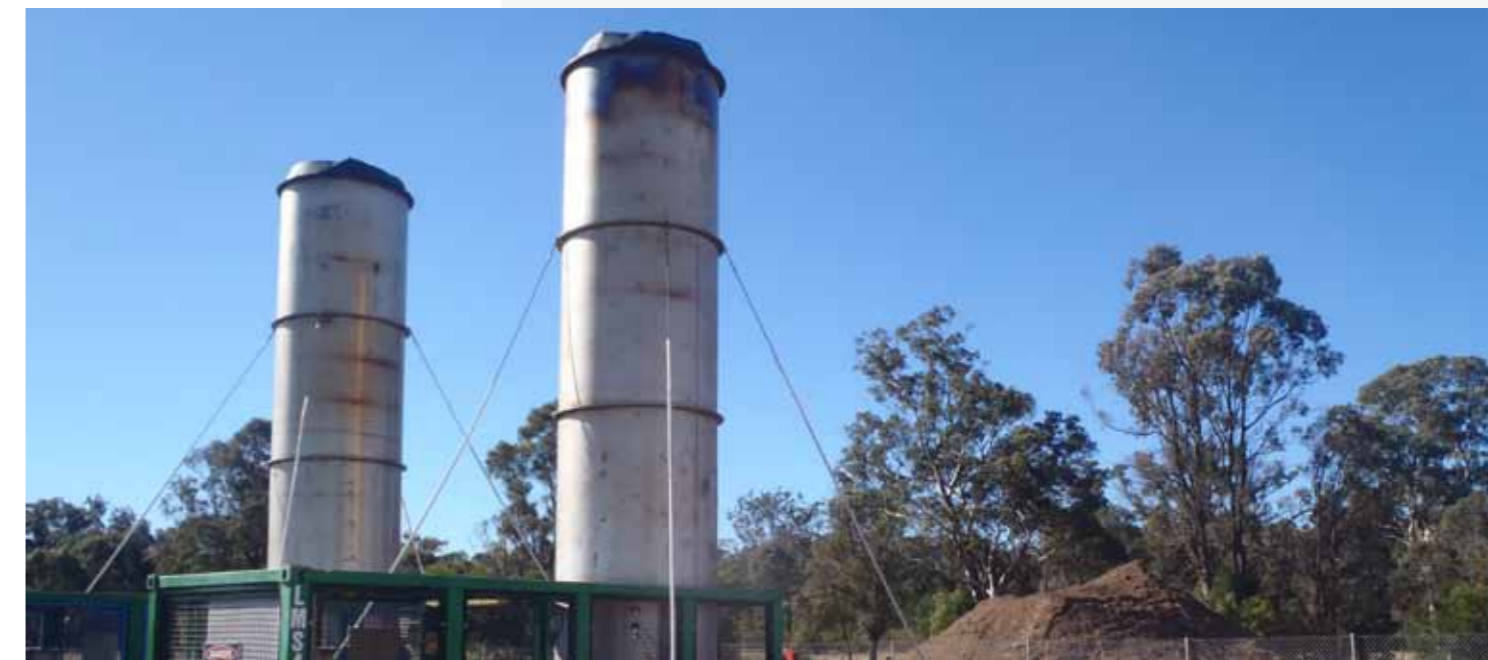
Where possible, Illawarra Coal utilises methane gas to generate electricity, however when this is not possible, the gas is flared in encased flare stacks, minimising greenhouse gas emissions and avoiding odour impacts.
