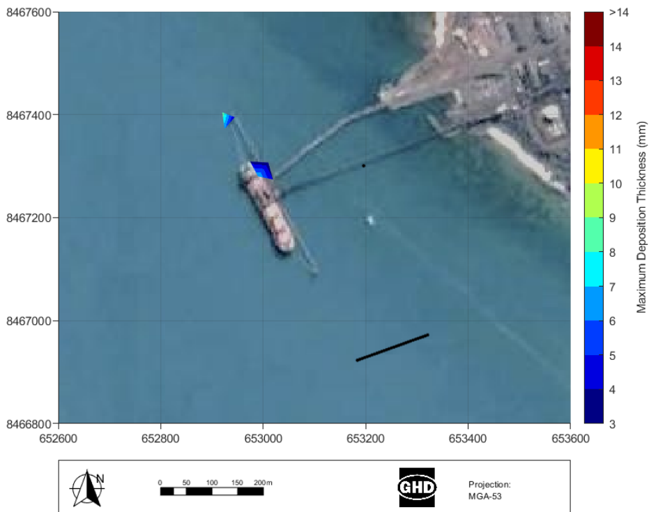
Figure 44 Maximum deposition thicknesses exceeding the Zol threshold of 3 mm, with STP outlet and diffuser ports shown in black
