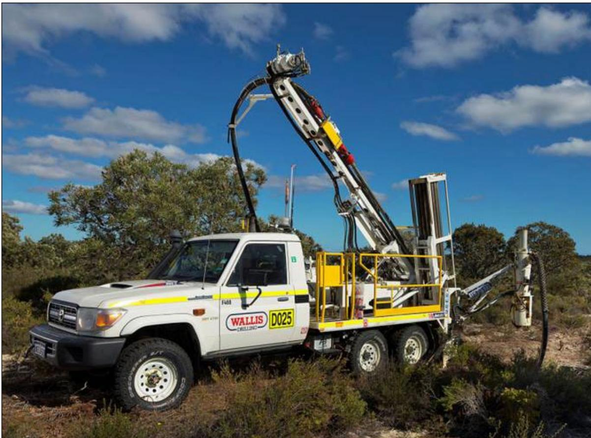
Plate 2-1 Example of a Low Impact Aircore Drill Rig
