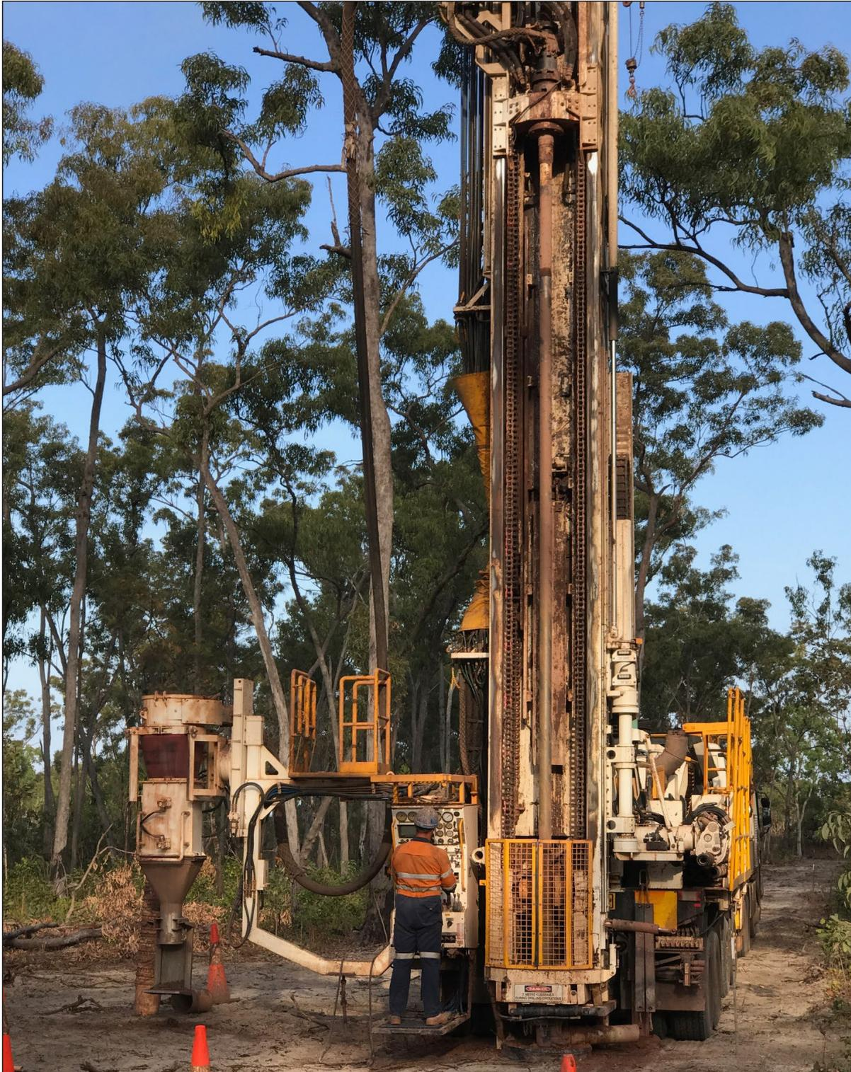
Plate 2-2 Example of a Reverse Circulation Drill Rig
