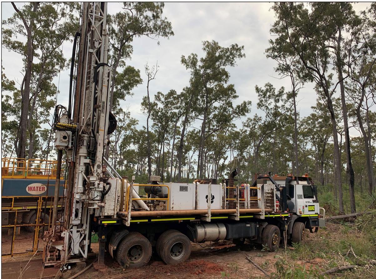
Plate 2-3 Example of a Diamond Drill Rig
