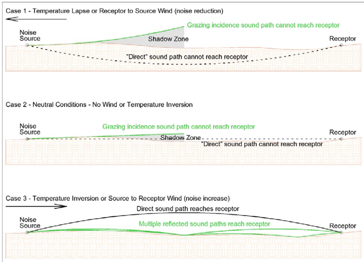
Where all sound paths intersect the ground or other structures rather than reaching the receptor, the receptor is considered to be in the shadow of a noise barrier and the received noise level is significantly reduced.
