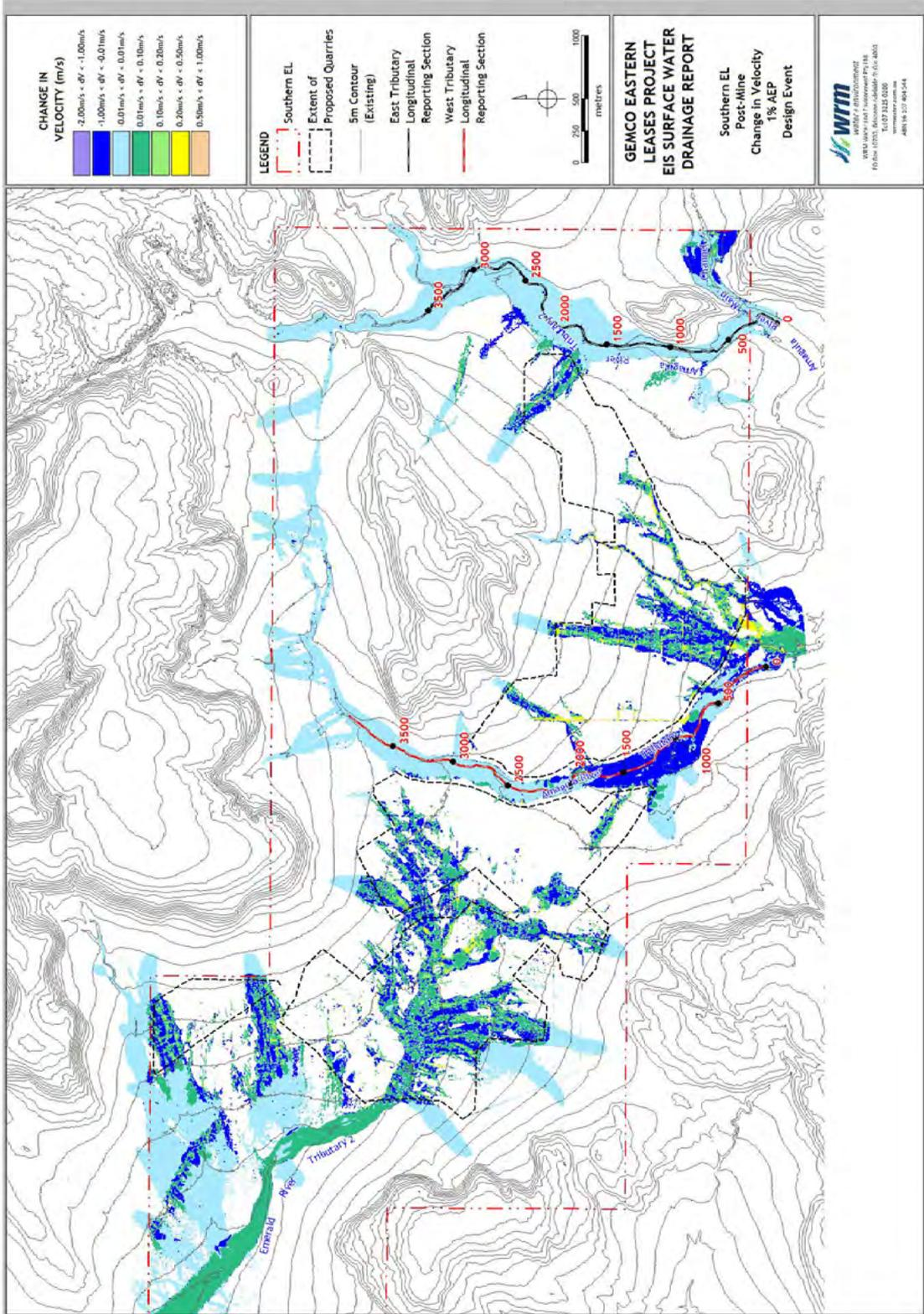
Figure 29 - Amagula River 1% AEP Post-Mining Change in Velocity
