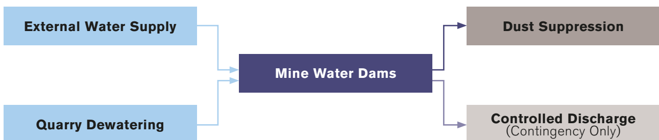
DIAGRAM 2 CONCEPTUAL WATER MANAGEMENT SYSTEM
