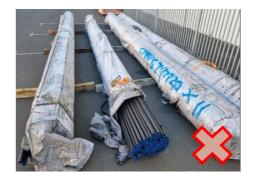
INSUFFICIENTLY STRAPPED WITH POOR STRUCTURE
