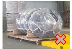
INSUFFICIENT FOR SIZE AND SHAPE - POOR STRAPPING AND NO SWL
