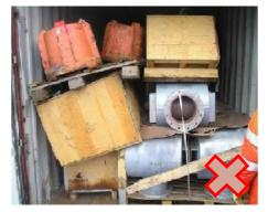
POORLY SECURED WITH HEAVY ITEMS ON TOP
