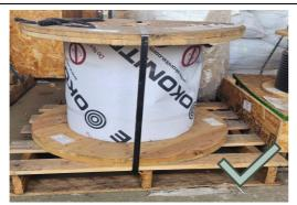
ON A CABLE REEL AND SECURED TO PALLET
