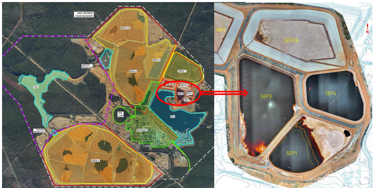
Figure 4: Solar Evaporation Ponds Configuration (including SEP1, 2A, 3 and 4)
